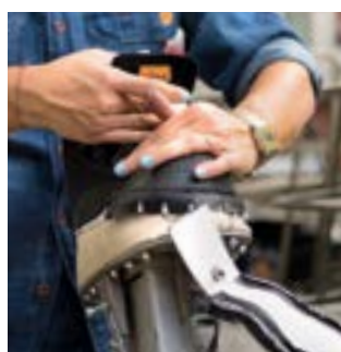
5 INSERIMENTO MEMBRANA WATER SHIELD Water Shield membrane insertion / Einsetzen Water Shield Mem- bran
